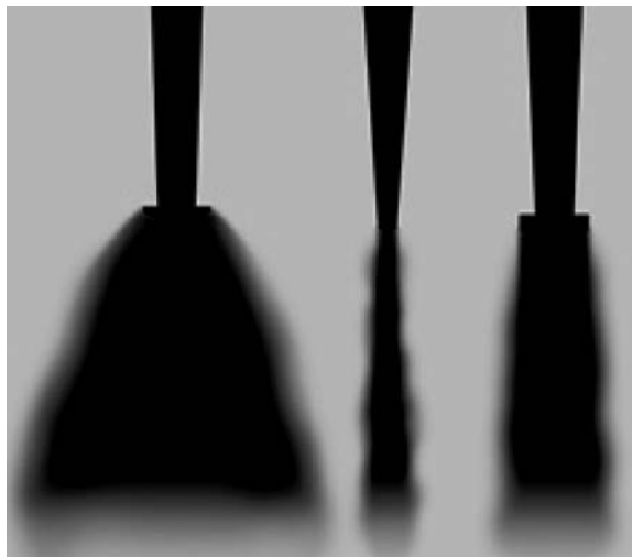
Figure 22.27 Different types of sprays obtained by ultrasonic atomization. (Courtesy of SonoTek Corporation)
