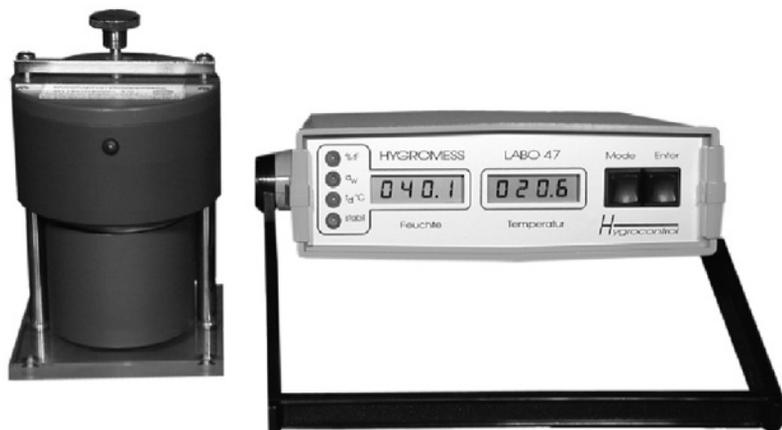
**Fig. 16.4** Capacitive humidity meter Hygrocontrol Labo 47 and a probe type 4703 for water activity measurement.
